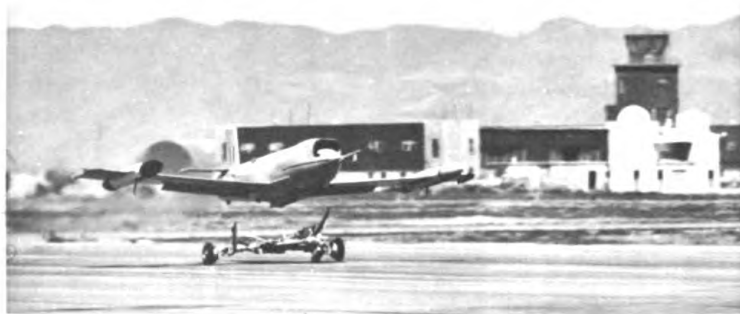
The Australian target Jindivik takes off from a tricycle trolley during a flight evaluation test at NMC.
