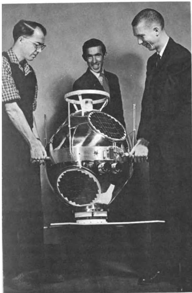
The Injun III satellite. Left to right, Curt Laughlin, payload manager; Dr. Brian J. O'Brien, scientist in charge; and Don Gurnett, project engineer. The VLF loop is at the top of the payload. The antennas are shown in the folded position for launch.
