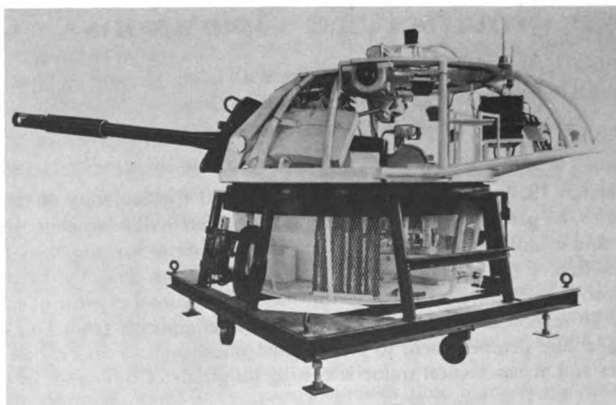
The M48A1 Tank Turret Trainer, Device 3A78. By means of this equipment, a tank crew learns to work together as a team in loading, turret maintenance, and operation of the M48A1 tank.
