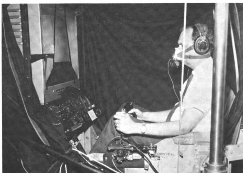
Figure 2 — The value of cockpit motion in alerting pilots to emergent conditions and in improving corrective responses is studied by means of a simulated pilot cockpit motion platform. Shown are the cockpit, controls, and visual display.
