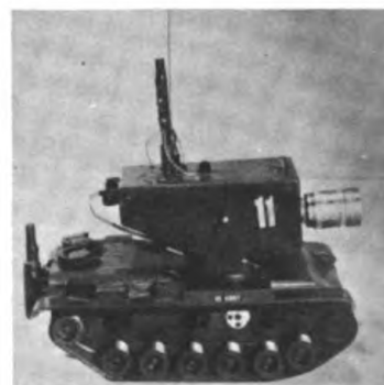
TV-controlled model tank; an element of the tank platoon-leader trainer.
