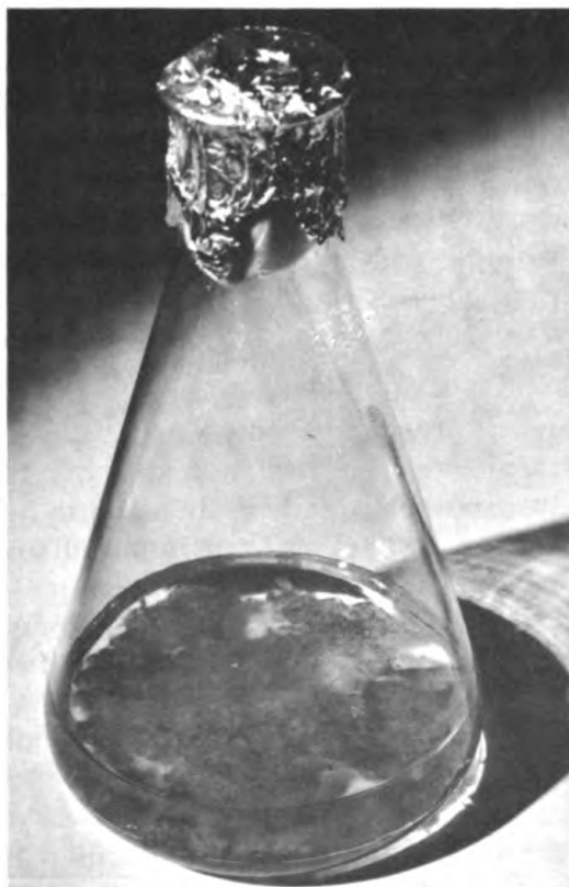
Figure 3 - Fungal mat growing at a fuel-water interface
