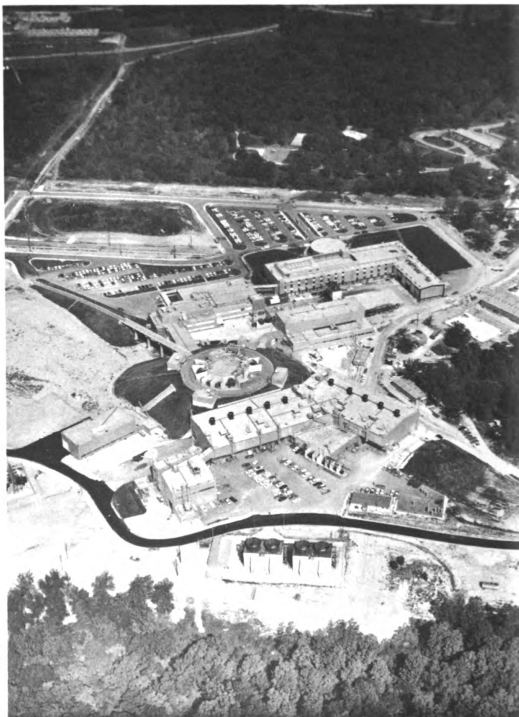
Aerial view of the Zero Gradient Synchrotron complex. The synchrotron is beneath the circular mound of earth at the center of the photograph.
