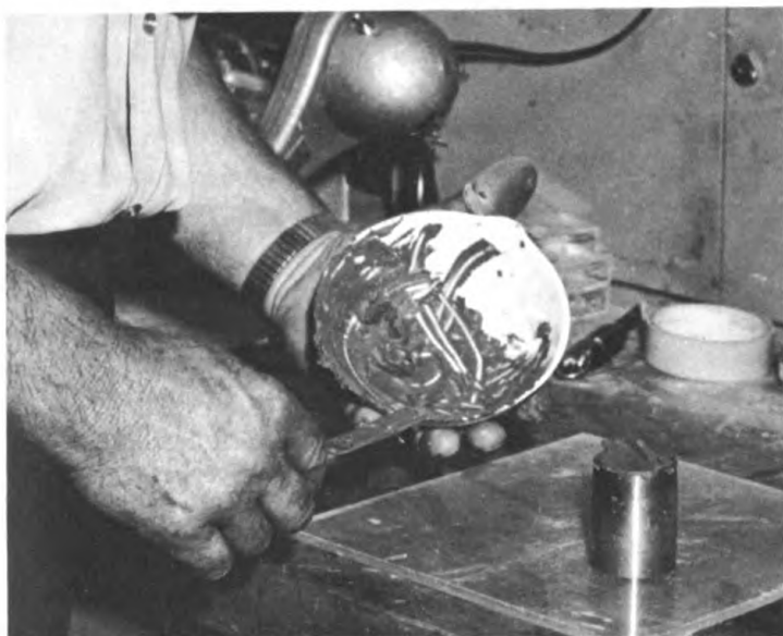
Fig. 6—Instrument used to study shear strength of soil samples.
