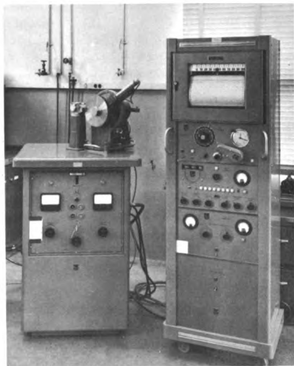
Fig. 5—X-ray diffraction test instrument used to study clay mineralogy. This instrument is required because samples are too fine grained for satisfactory microscopic study.
