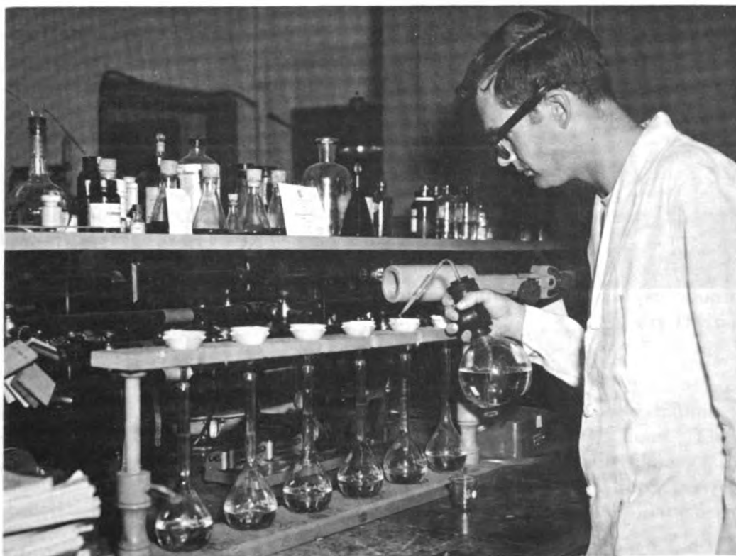
Fig. 4—A technician analyzes the carbonate content of a soil sample.
