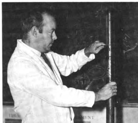
Fig. 2—NCEL scientist strips protective wax coating from ocean-floor soil sample preparatory to analysis.
