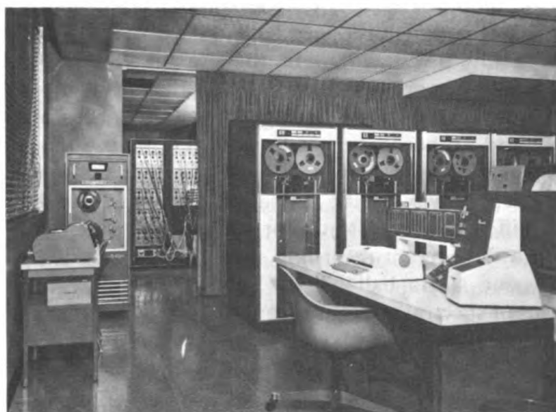
Figure 7 - Another view of the IBM 1410 data-processing system, showing its relation to the 50 pre-amplifiers and an off-line magnetic-tape digital plotting system, at left, used for the preparation of curves. The black-out curtains provide a semi-dark area in the background for photographing signals on the cathode-ray tubes.
