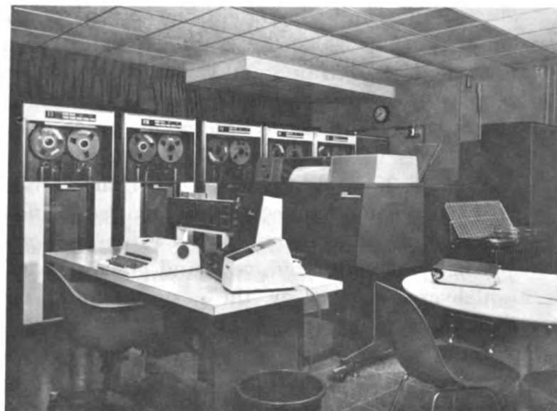
Figure 6 - View of the IBM 1410 data-processing system, showing the five tape drives. The magnetic tape drive, at left, can be connected to the telemetry system of Figure 4 to transfer data to the data-processing system.
