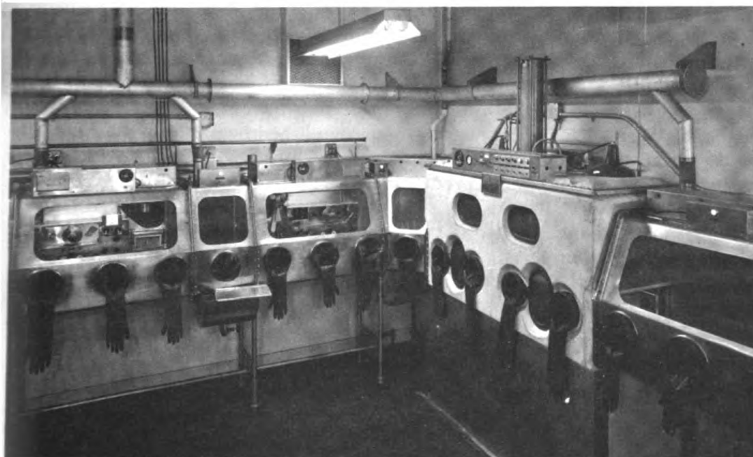
A completely sealed system used at NBL for handling infectious material which readily becomes airborne.
