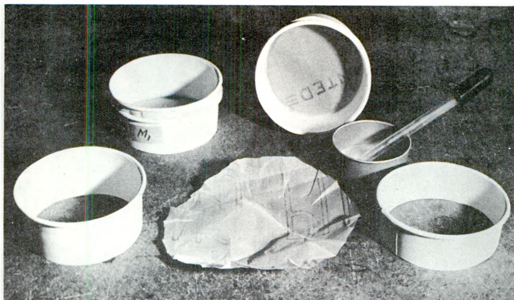
Non-metallic bolting-cloth sieves. In front, sieve components (paper hoops, bolting cloth, and wax). In rear, finished sieves.
