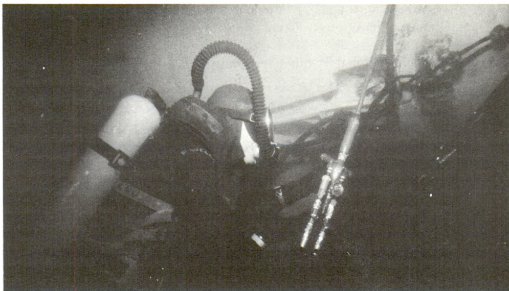
Aquanaut Paul Wells sprays foam into an aircraft hull to provide buoyance required to raise the object to the ocean surface.
