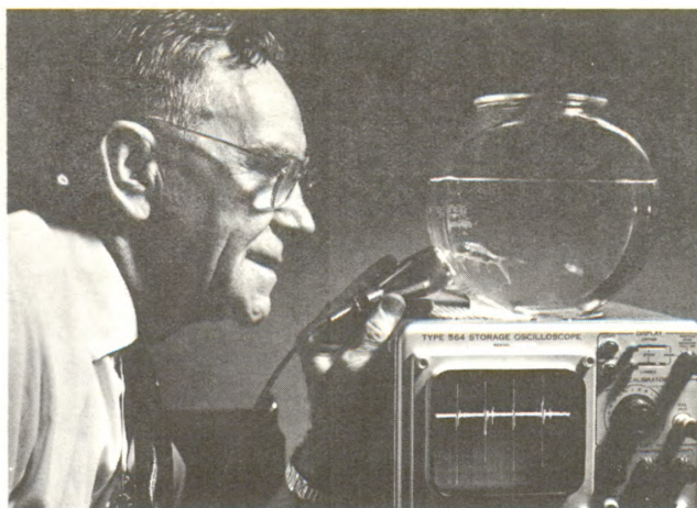
Mr. Richards, inventor of the UDC, demonstrates his ultrasonic transmitter and receiver. The device can monitor many kinds of movement, including respiratory activity of a goldfish, as shown in the photograph, the heartbeat of an unborn child, and the pulsations of blood in veins.
