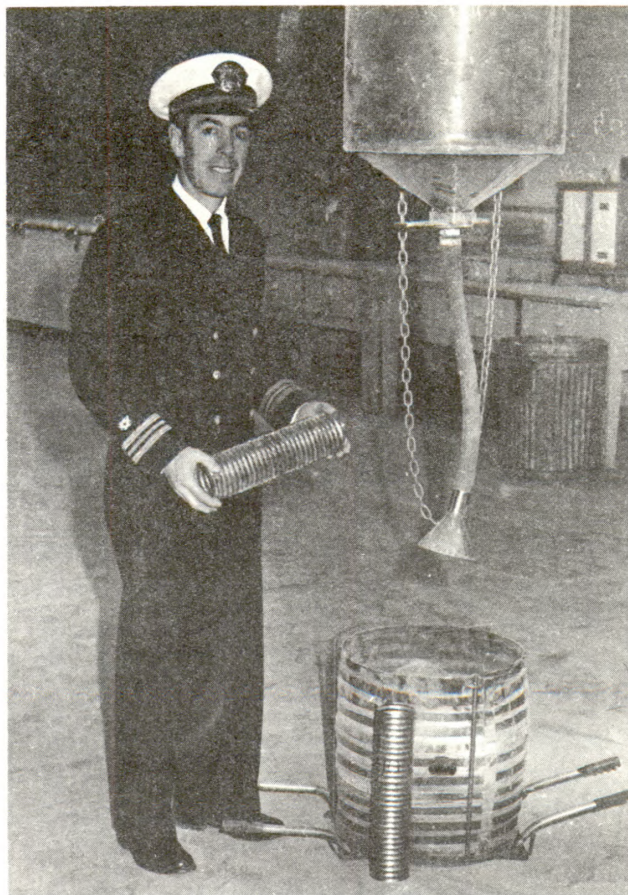
LCDR Watkins holds model section of corrugated conduit. Beside him is equipment used to test load-carrying capacity of models.
