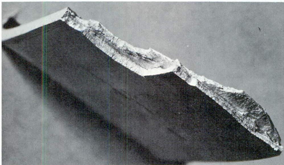
Figure 2 — Aluminum structural member that failed as a result of embrittlement by liquid gallium.
