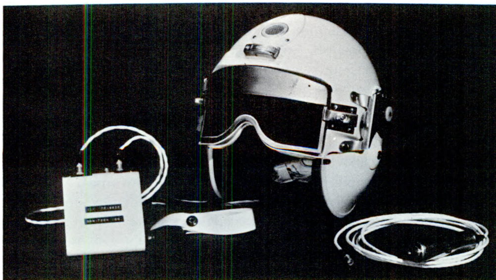
Figure 1 — An APH-5 helmet that has been modified to accommodate a visor designed to protect the wearer from intense visible radiation.
