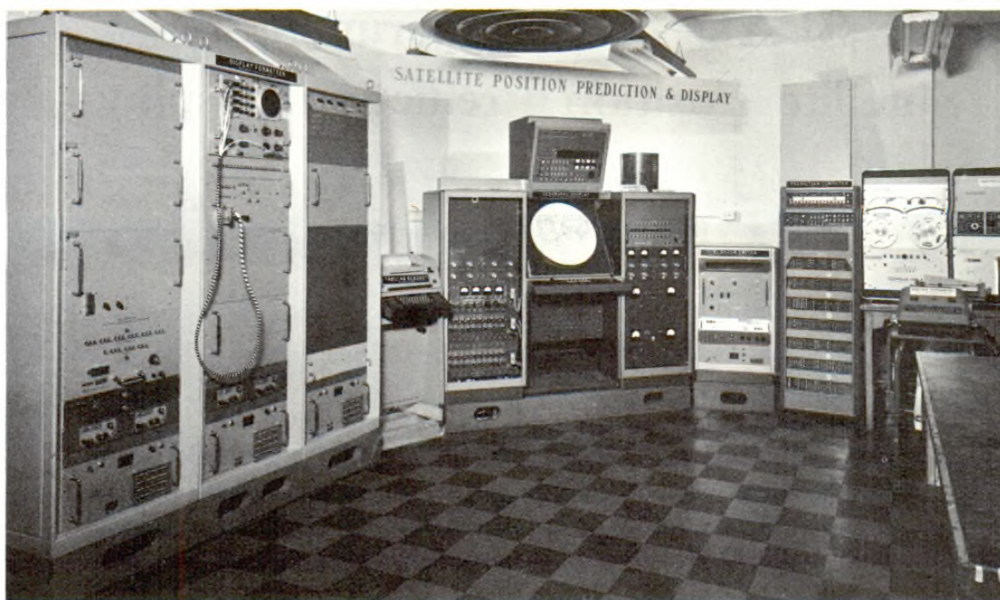
Figure 1 — Complete SPAD equipment as installed at the Naval Research Laboratory. The AN/UYK-1 computer (extreme right) feeds received data to the formatter (extreme left), which converts it to a form suitable for display. Tabular readout is at left of display console.
