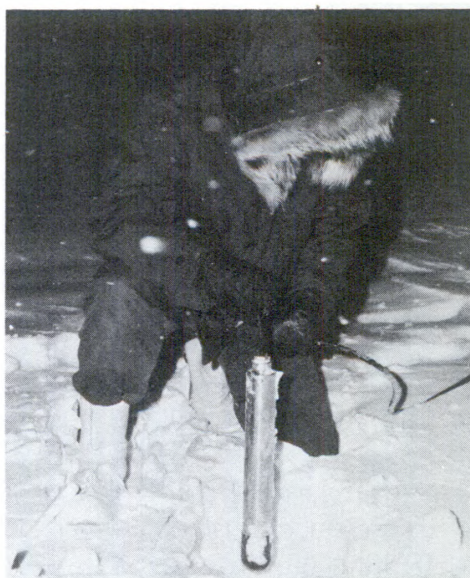
A hydrophone is lowered into a hole in the ice of ARLIS II to record echoes produced by explosions.
