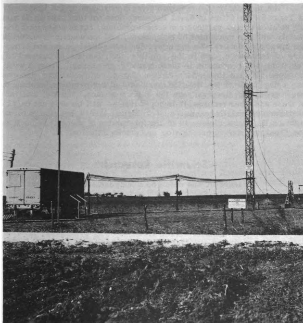
Fig. 10. A closeup of the University of Texas micrometeorological research site. The van at left houses the amplifying and recording equipment.
