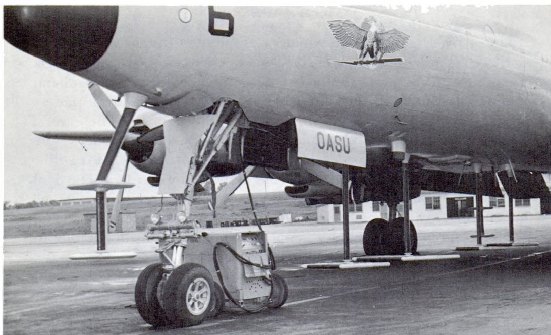
A view of the antenna installation showing a high-band, double-bay, co-linear array mounted forward of the nose wheel and several low-band hayrake antennas mounted in-line on the underside of the fuselage.
