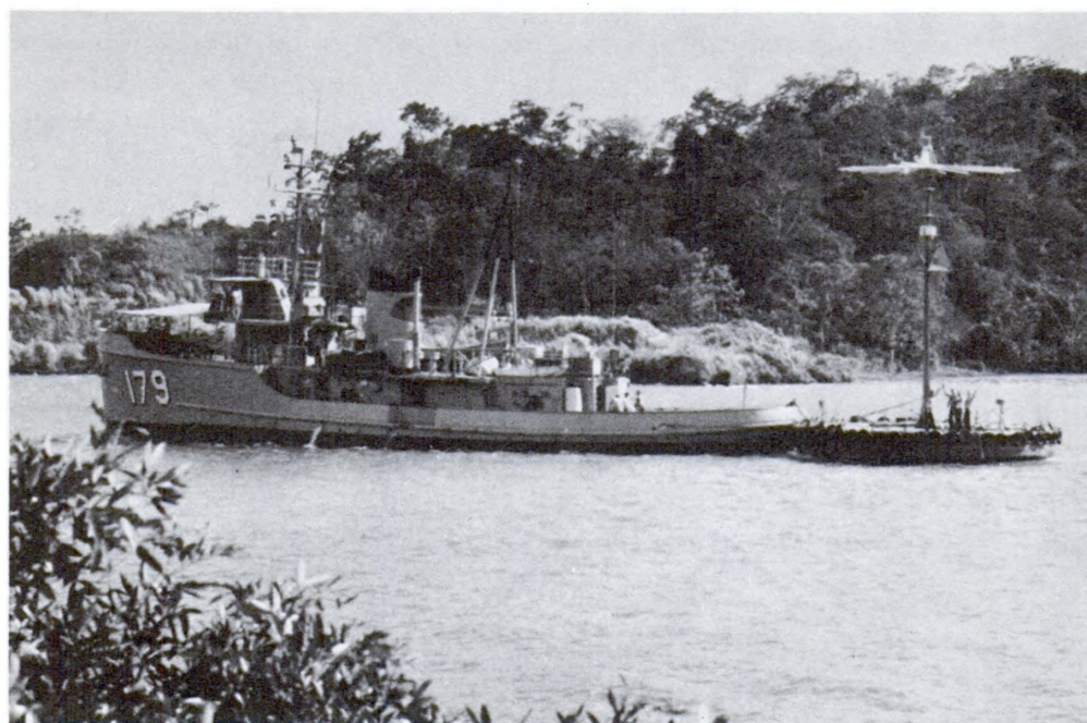
The Monster Buoy, the Navy's first experimental ocean data station buoy, is towed through the Panama Canal on the way to its home base in San Diego. Developed for ONR by Convair, the buoy is designed for operation at sea for one year without maintenance.
