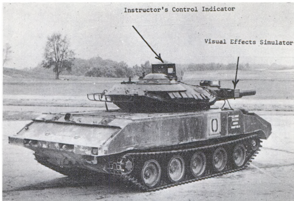
The Sheridan Weapon System (Device 3A101) trains gunners in the operation of the Shillelagh missile system
