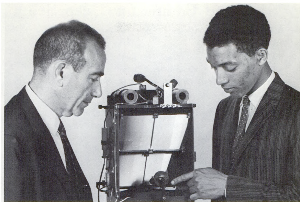
Dr. George R. Carruthers (right) and Dr. Herbert Friedman, shown with image intensifier ultraviolet spectrograph which Dr. Carruthers developed for the Aerobee rocket.
