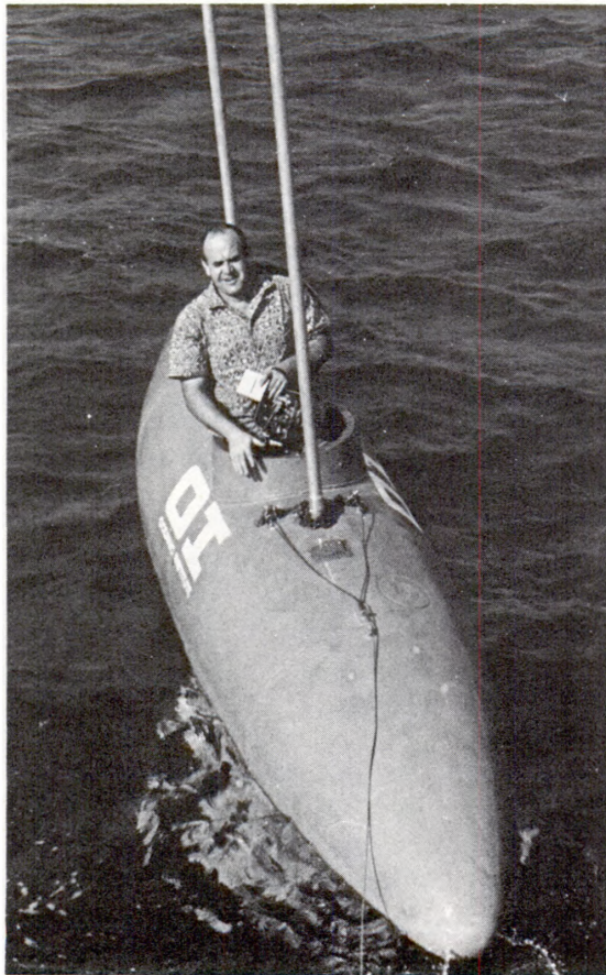
Ken Norris and his Mobile Observation Chamber, a converted jet gas tank. Vertical pipes serve as breather and antenna posts.
