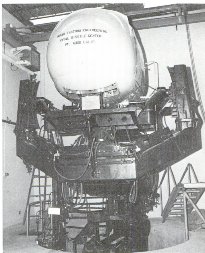
Figure 4 — View of the dynamic-base cockpit used in the VCAD Evaluation Program
