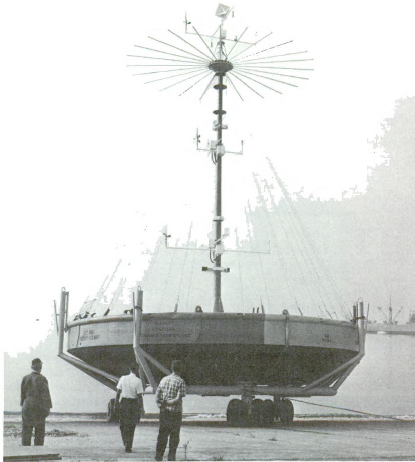
Convair-developed "monster buoy" is 40 feet in diameter and 7-1/2 feet deep
