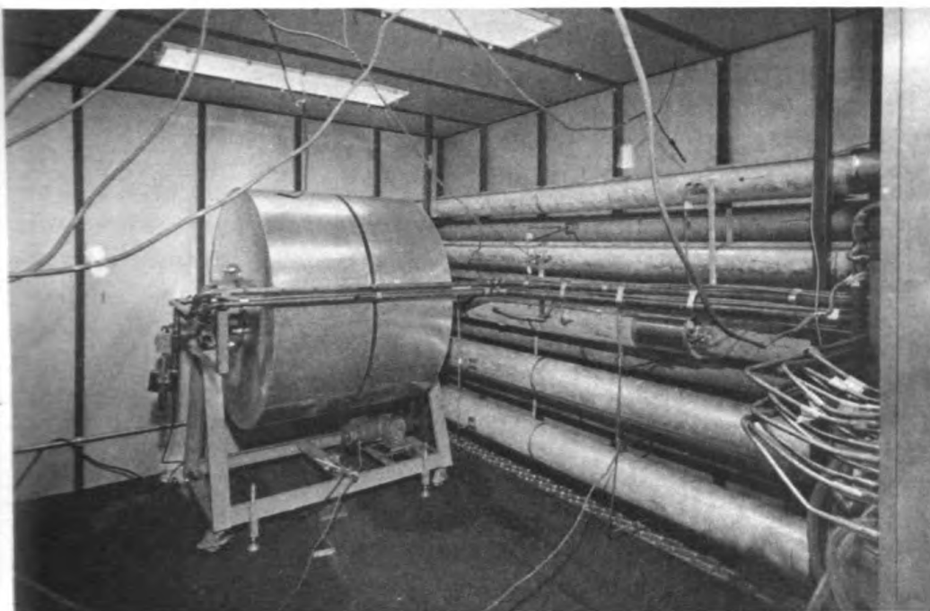
Two 500-liter roller drums and dual aerosol transport apparatus, housed in room with controlled temperature and humidity
