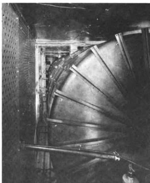
Eight roller drums of 1500-liter capacity. Drums are located in rooms with controlled temperature, humidity, and air flow.
