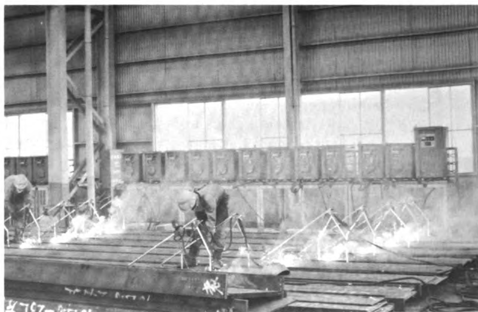
Figure 5 — Multiple gravity welders operated by single workman in continuous operation
