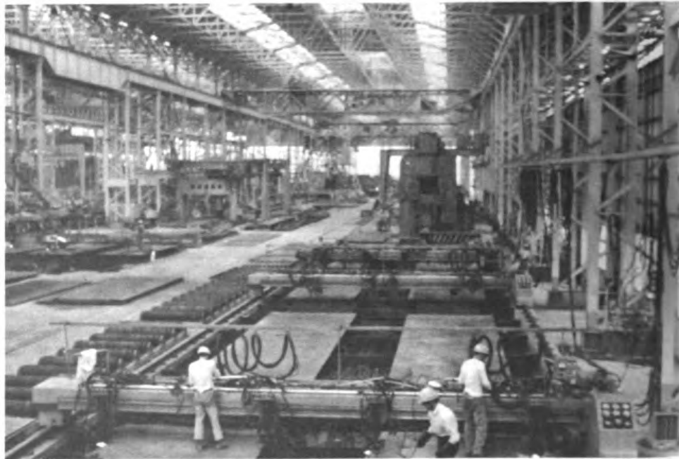
Figure 3 — Flame cutting and steel fabrication. Note large aisles and buffer areas and small number of workmen during normal operations.
