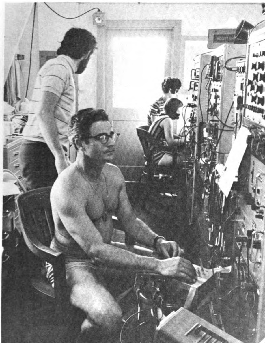
Figure 4 — Tape recordings of stimuli used in underwater sound localization experiments are randomly presented (foreground) by the experimenter. Assistants (background) monitor divers' responses as they are recorded on an IBM key punch.
