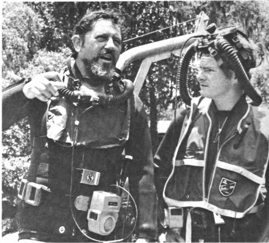
Figure 2 — Divers wearing Bioengionics muzzle (left) and U.S. Divers mask (right). These units are two examples of the various types of masks/muzzles/helmets used by the Communication Sciences Laboratory in underwater speech intelligibility experiments.
