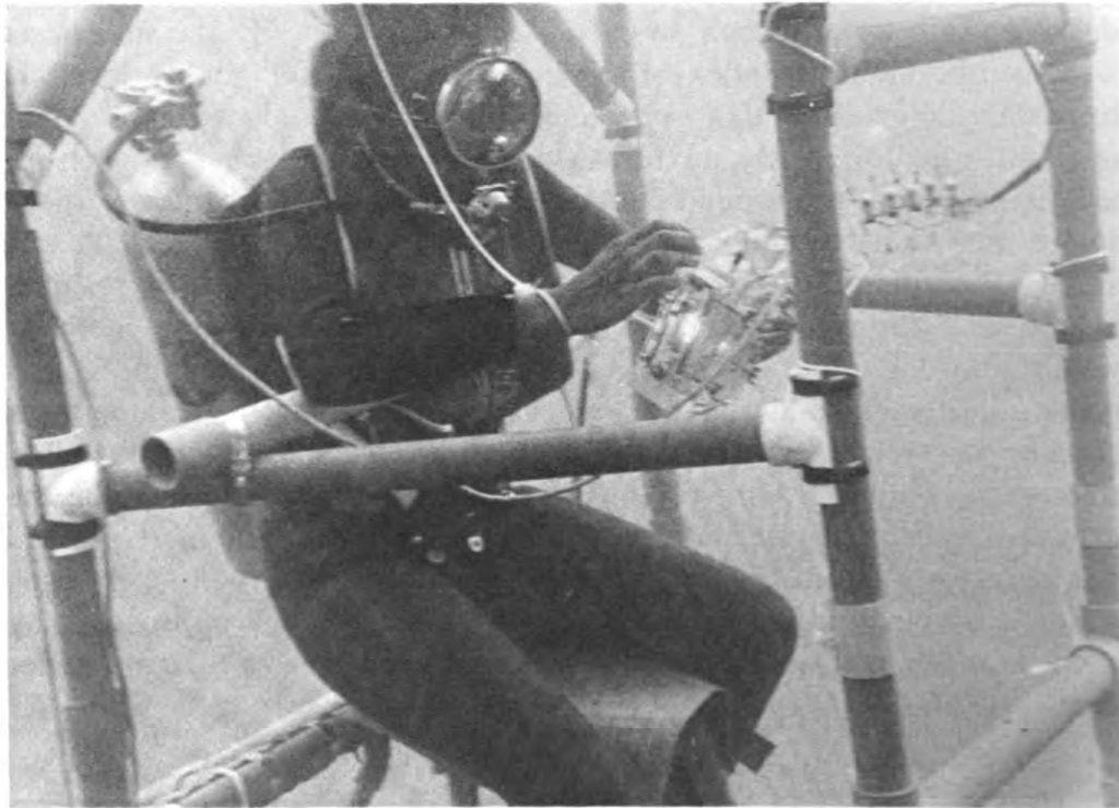
Figure 3 — A diver/subject seated in DALS (Diver Auditory Localization System) and responding to acoustic stimuli in an underwater sound localization experiment. The diver's response is recorded on surface equipment via an underwater switching apparatus.
