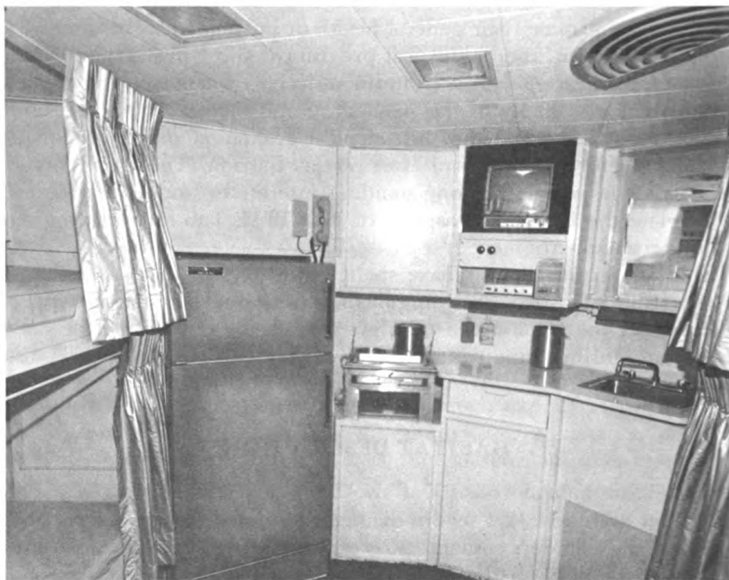
Interior view of crew quarters shows bunks for the four aquanaut-scientists, the entertainment console, and galley. The crew will live 60 days continuously below the water's surface using the GE designed and built habitat as home and laboratory.
