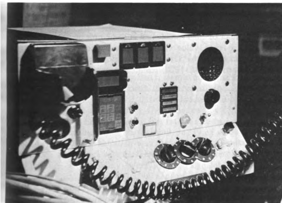
Experimental digital signaler under evaluation by Destroyer Development Group II
