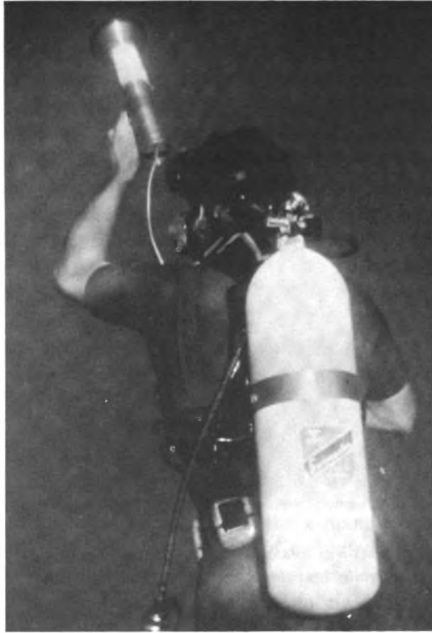
Aquanaut using sonar gun to locate lobsters which had been tagged. Because of the tag the sonar could pick up the lobster thus supplying data for studying his movements.
