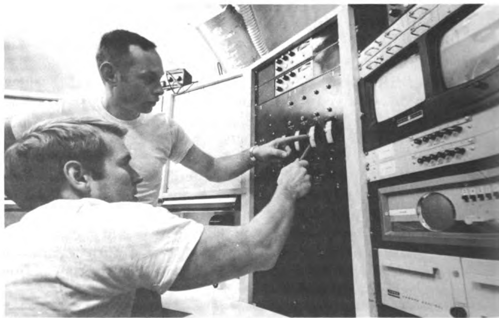
Mahnken and Clifton using mass spectrometer which monitors the atmosphere of the habitat. A similar spectrometer was located in the surface support van.
