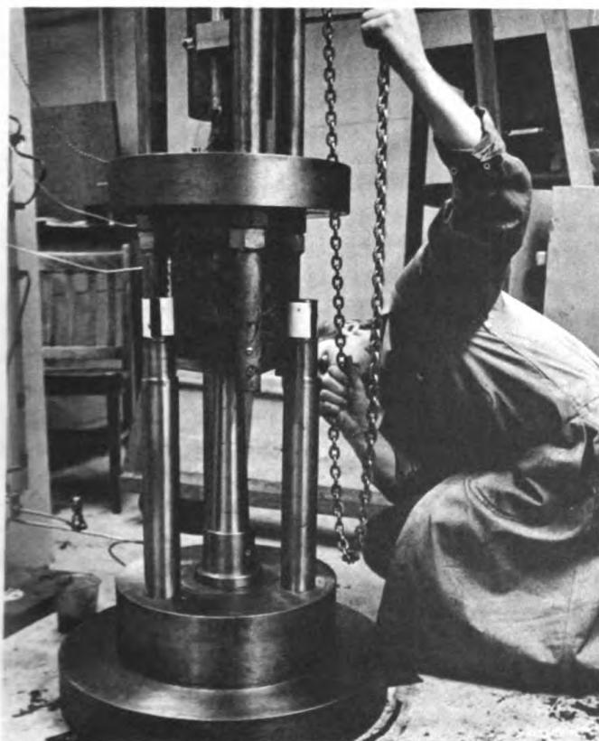
Figure 8(b) - The operator carefully lowers the upper half of the press assembly onto the tapered pressure chamber (center) and the surrounding supporting posts. The two heavy constraining rings (only one visible in this picture) and the high-pressure plunger housing.
