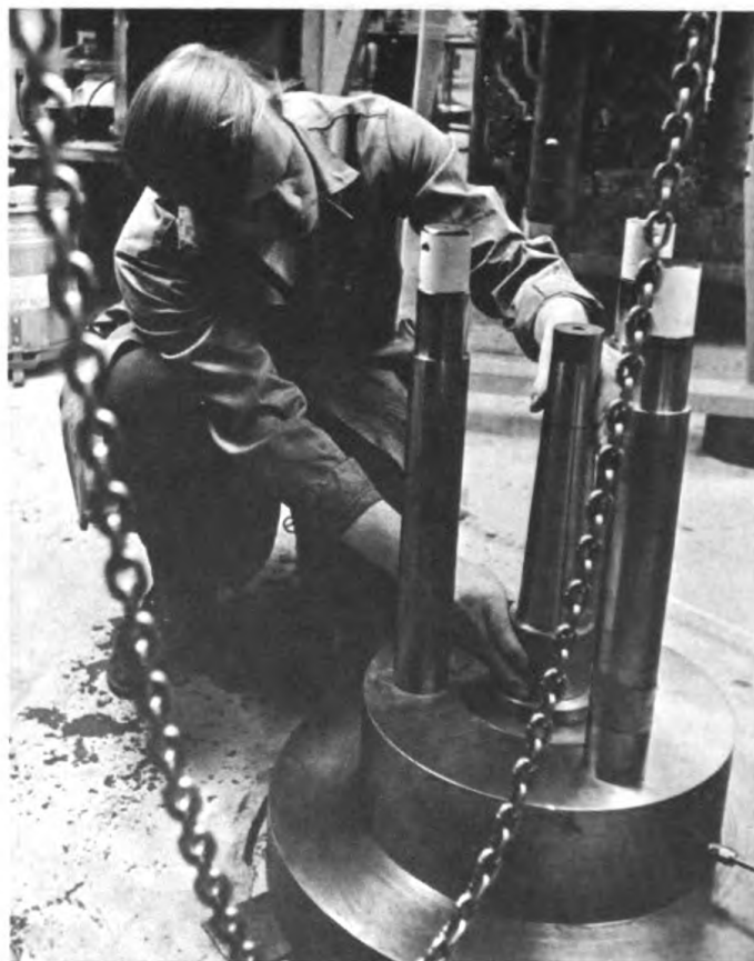
Figure 7 - After assembling the internal components (see Figure 3), the operator places the tapered high-pressure chamber in position to receive the constraining rings and piston from above
