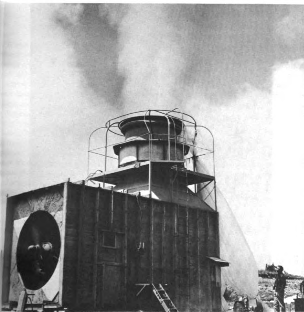
Apparatus for artificial production of atmospheric space charge in concentrations similar to that found in thunderstorms
