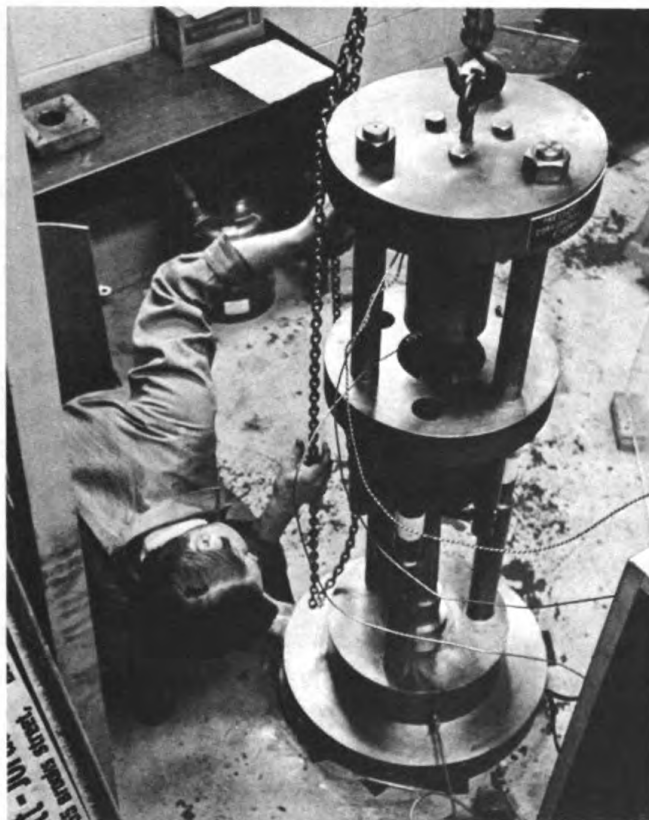
Figure 8(a) - The operator carefully lowers the upper half of the press assembly which consists of the two constraining rings and the high-pressure plunger housing, onto the pressure chamber. Tubing carrying the pressurizing fluid can be seen entering the plunger housing located between the two constraining rings. Visible at the extreme lower part of the picture is tubing carrying the back-pressure fluid for the other plunger located in the base of the press.
