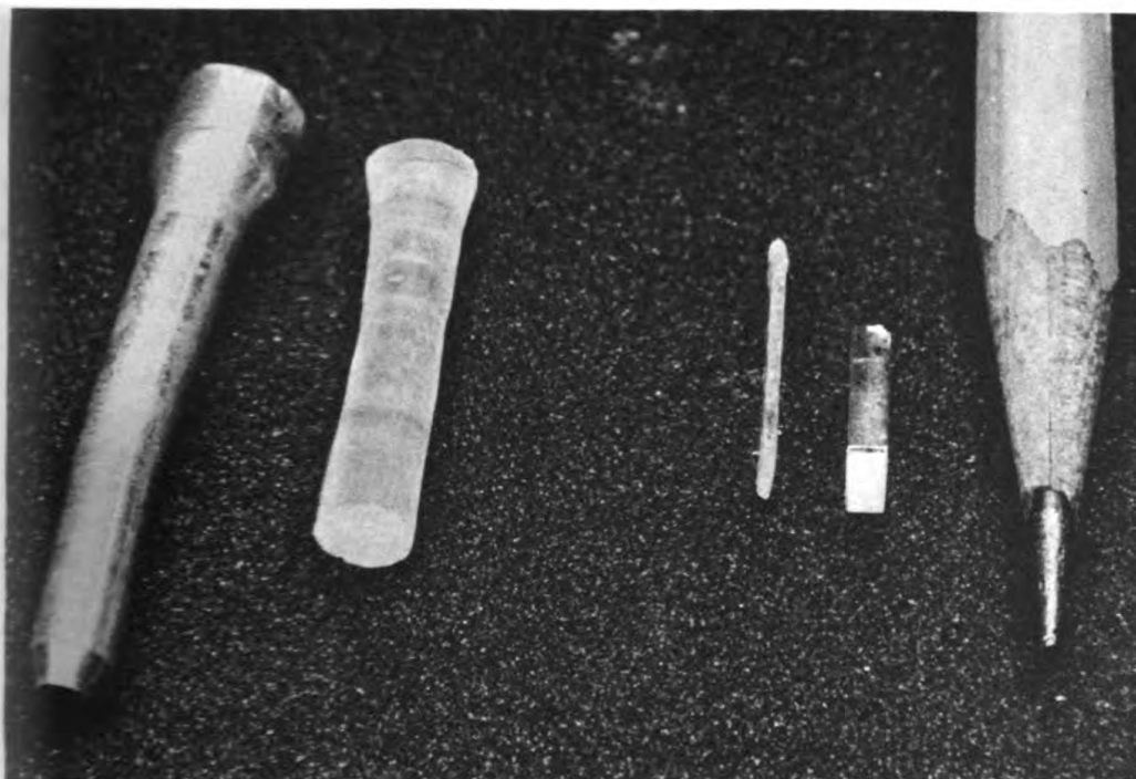
Figure 5 - Examples of extrusions produced in the Northeastern University experiments. The pieces are (from left) partially extruded aluminum; partially extruded cylindrical salt crystal; extruded sheet of salt crystal and sheet of salt crystal before extrusion. Pencil at right shows relative size of objects.
