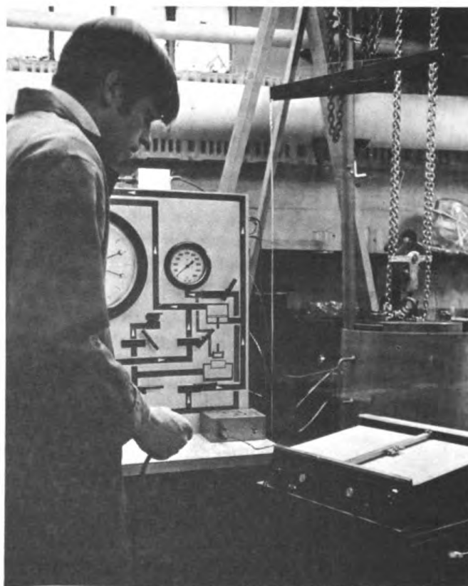
Figure 9 - As the pressurizing process begins, the operator makes adjustments on the control console. The X-Y recorder is at the right while the top part of the pressure chamber is visible in the background beyond the protective shield of plexiglass. The flow pattern of the pressurizing fluid is outlined on the face of the console. A schematic diagram of the top and bottom plunger is shown on the right side of the console.
