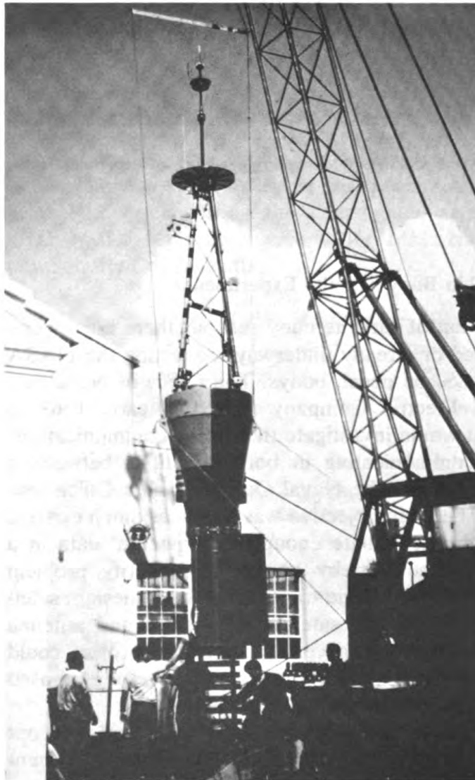
Figure 4 — Shown here is a Sea Robin Buoy that is 14 feet long, 4 feet in diameter at the top, sloping to 2 feet in diameter at the mid section. The buoy in its initial configuration weighed approximately 1500 pounds.
