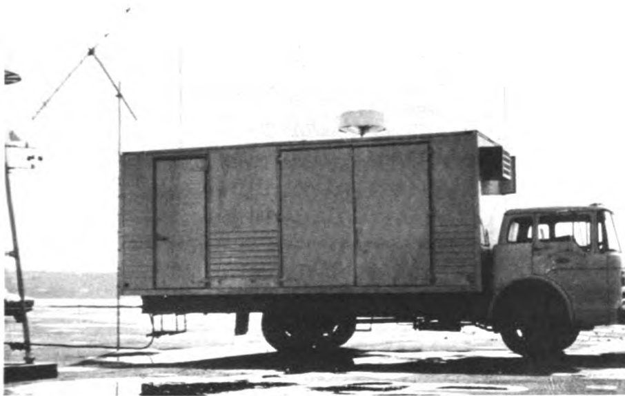
Figure 6 — The sensor read outs of the Sea Robin are transmitted via UHF link to the General Electric developed van seen here
