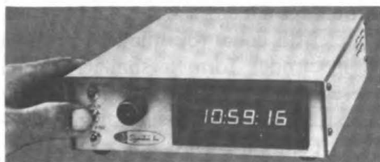
Figure 5 — Digital clock using LEF seven-segment numerics
