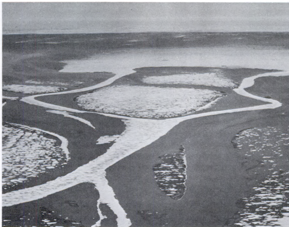
Figure 2 — The prebreakup floodwaters flow over the areas of bottom-fast ice and cause the areas of floating ice to fluctuate up and down with stage
