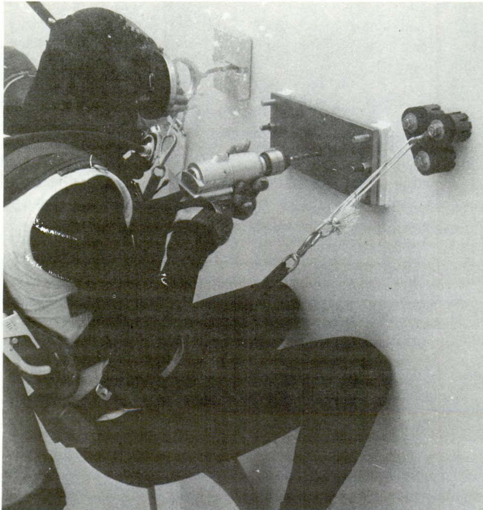
Figure 4 — Underwater tasks involving use of torque require systems that can counteract forces developed in the weightless environment. The diver shown above is drilling underwater while making use of what appears to be a restraining device held firm by magnetic clamps. The problem of force counteraction is encountered in the outer space environment also, and similar devices are under development to solve those problems. Note heavy gloves required to keep diver's hands warm.
