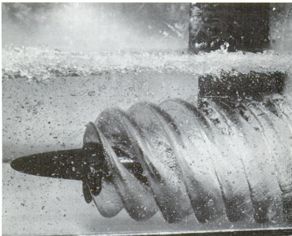
Figure 1 – Vortex cavity behind a super cavitating propeller is shown in this photograph. The invention of super cavitating propeller is one of most significant technological achievements during last decade in the field of high speed hydrodynamics. In spite of its many distinct advantages, the material problems and cavitation erosion are still limiting its widespread use.
