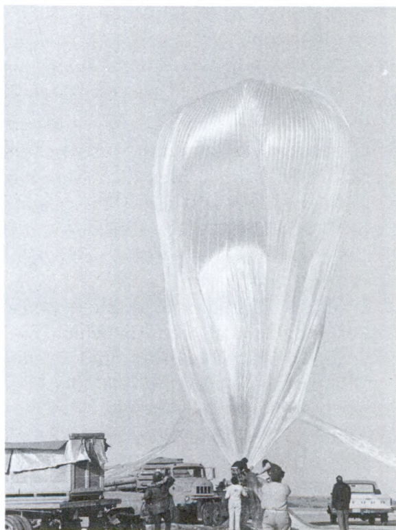
Figure 7 — Inflation of the balloon bubble with helium gas
