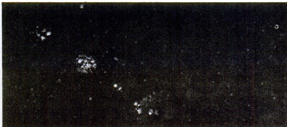
Figure 2 — Photograph of transient cavitation. Here the stroboscopic flash interval was 2.4 msec, the acoustic pressure amplitude at the antinode was 4.7 atmospheres, and the maximum velocity achieved about 100 cm/sec. The diameter of the largest cavity was approximately 1 mm.
