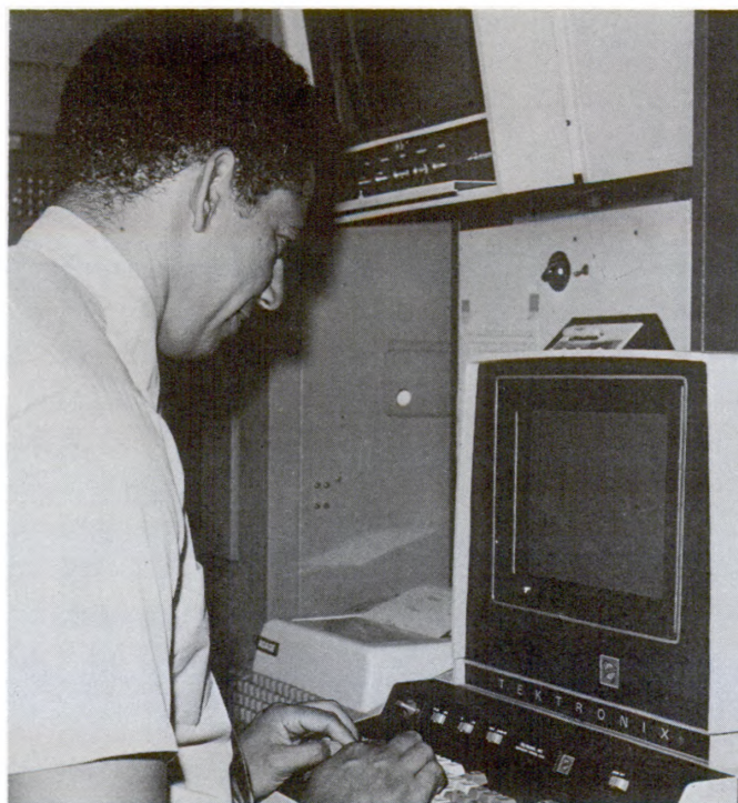
Figure 12 — Don Robinson, an electronics engineer at NUC, punches in a program for a run of the Mark 48 torpedo. The television screen above him will give him a visual presentation of the torpedo run on a target.
