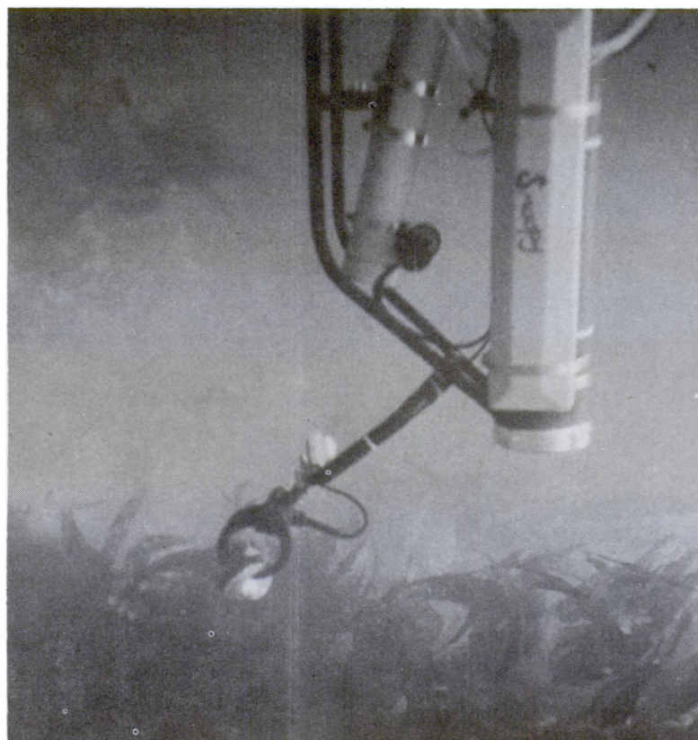
Figure 9 — Snoopy picks up a large seashell in about 50 feet of water off Catalina Island in a recent operational test of its new capabilities. In addition to the new grabber seen in this photograph, the vehicle now has a compass and automatic depth control.
