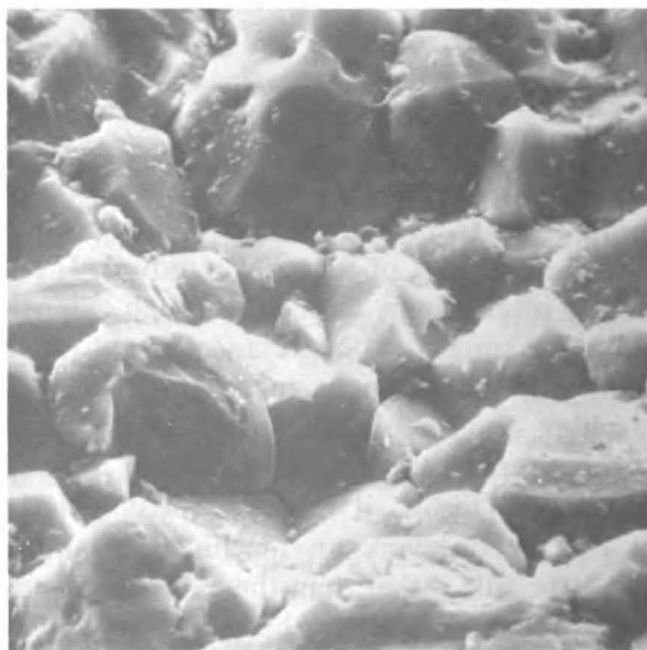
Figure 5 – Scanning electron micrograph of sintered polycrystalline Ni-Zn ferrite ground with a 100 grit diamond wheel. In a ceramic with low impact resistance, material removal occurs mainly by brittle intergranular fracture. Grinding direction – horizontal.
