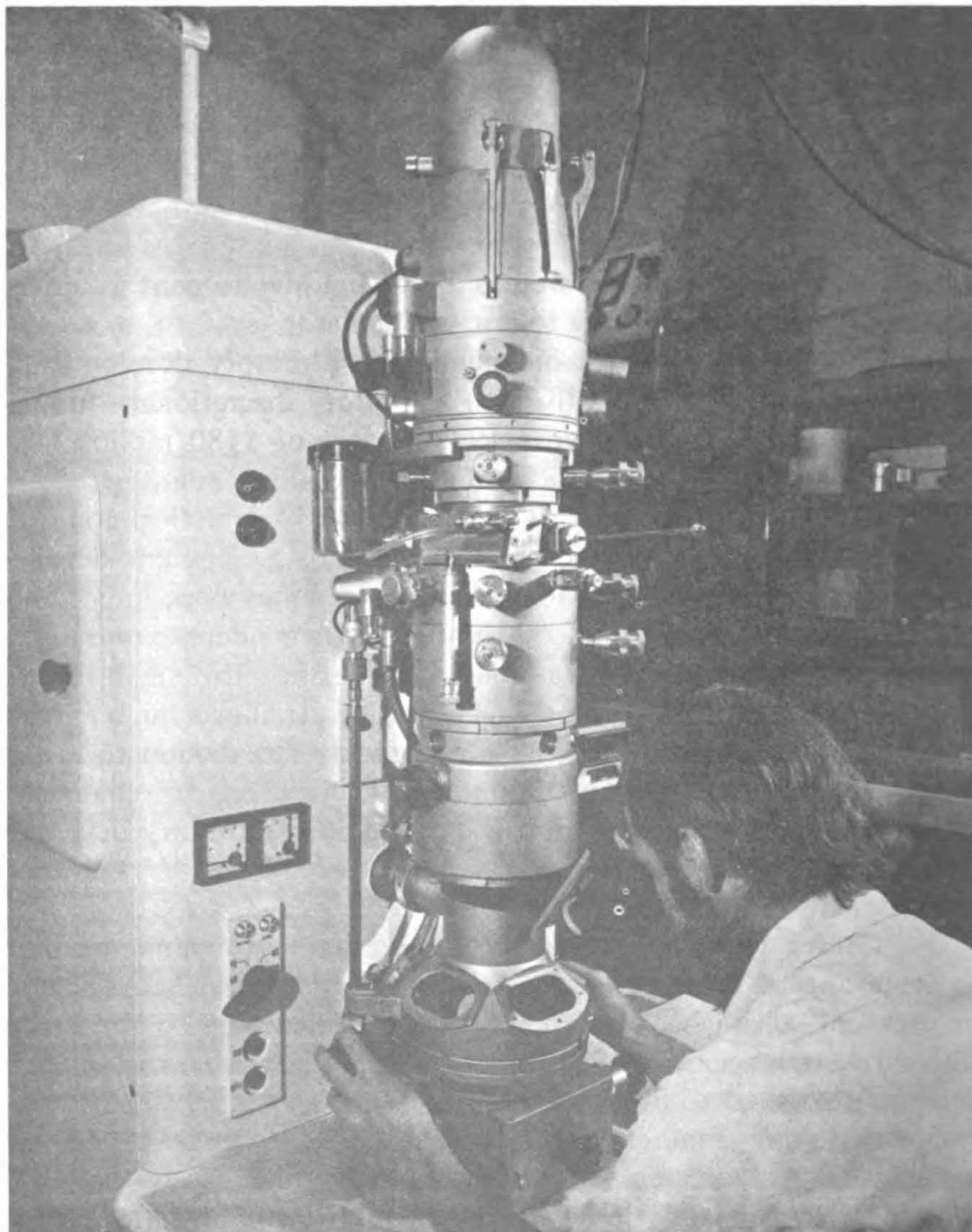
Figure 5—Transmission electron microscope used for a study of the internal structure of metals
