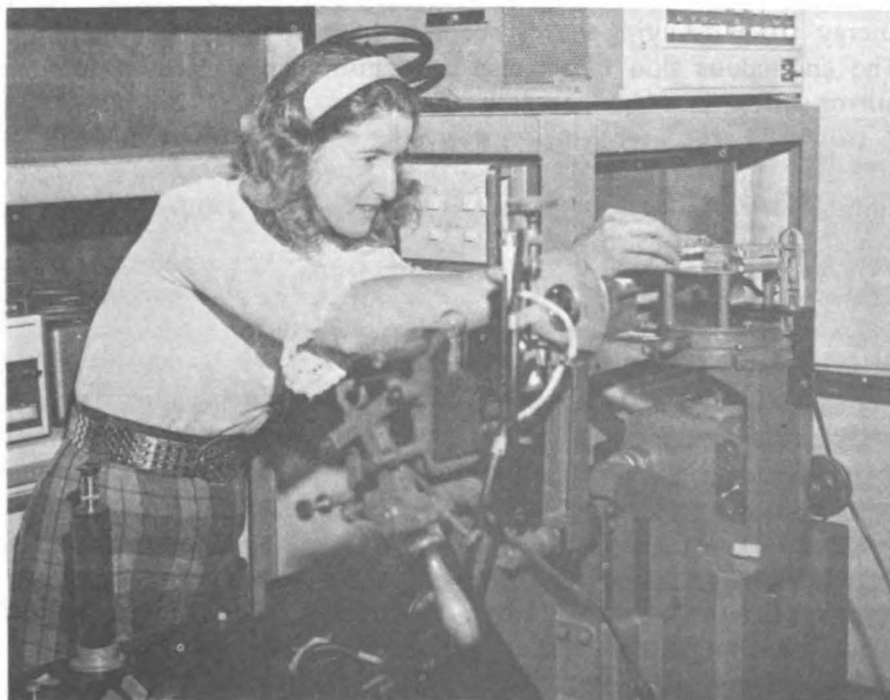
Figure 3—Jean Bennett adjusts the interferometer to obtain sharp interference fringes contouring the irregularities on a mirror surface
