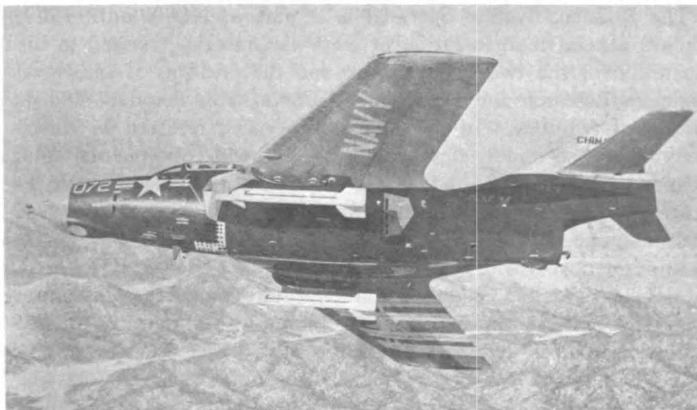
Figure 2—Sidewinder, the nation's first passive infrared-homing air-to-air guided missile, on F-9F aircraft. This photograph was taken in 1956, the year Sidewinder was released to the Fleet.
