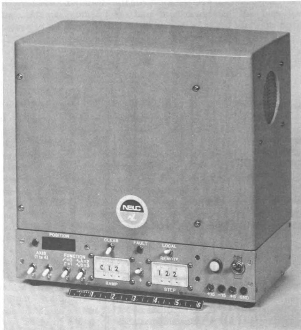
Figure 3 – The Advanced Development Model (ADM) minicontroller has been tested on a number of operational systems, including a Mk 42 Mod 9 5"/54 gun located at the Naval Weapons Laboratory.
