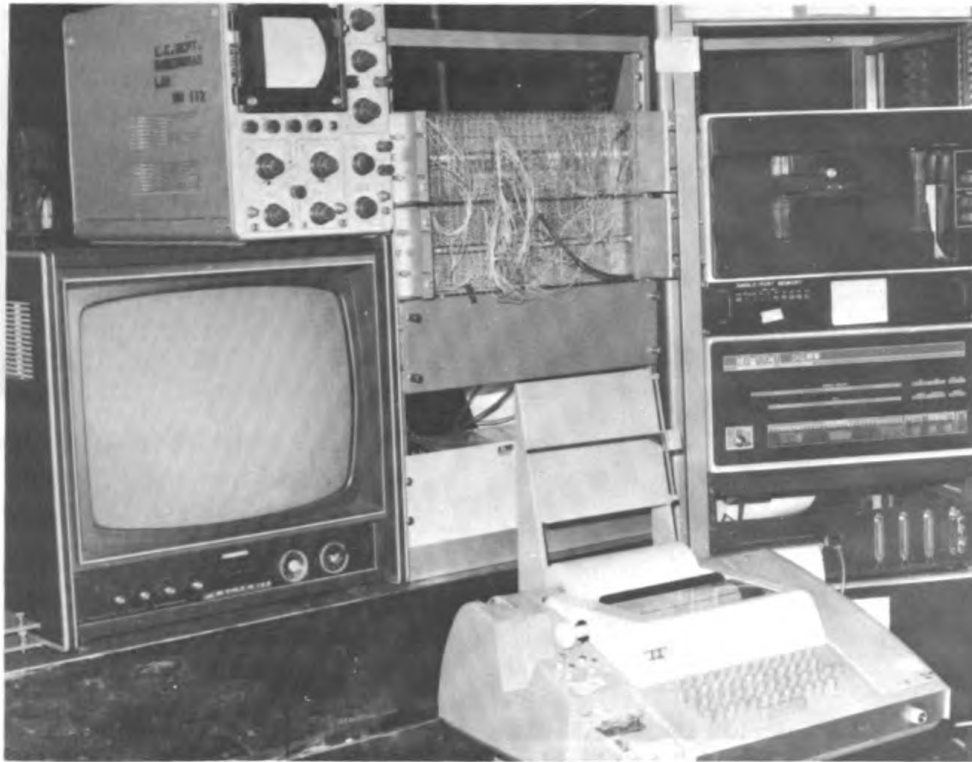
Figure 4 – Digital section of the programmable optical processor.
