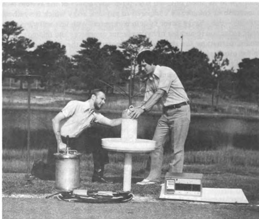
Displaying the components that make up the environmental sensor package being developed at NCSL. The remote sensor will provide on command real-time data on water current, water depth, and surface wave height and wave period.
