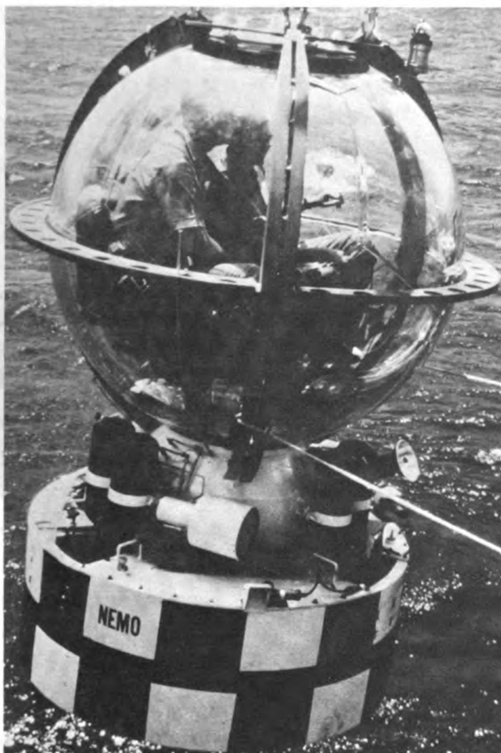
Figure 2 — CEL's NEMO (Naval Experimental Manned Observatory) can carry two men to a depth of 600 feet. Constructed from 12 acrylic plastic pentagons bonded together to form a sphere, NEMO provides full 360 degree visibility.
