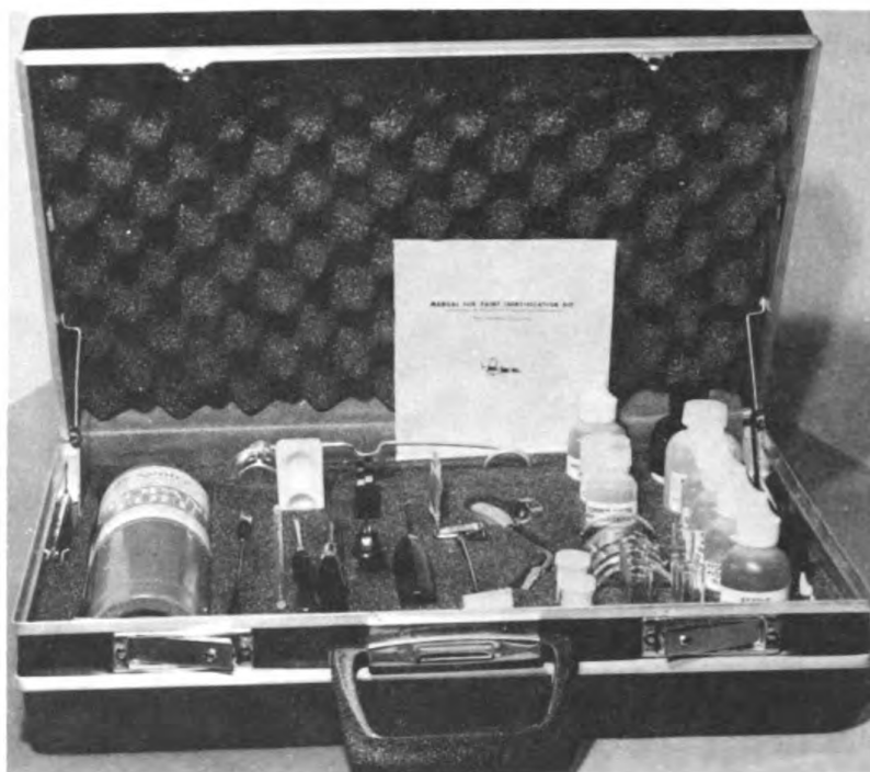
Figure 5 – The CEL-developed weathered paint identification kit for field personnel with no laboratory training. It is now being manufactured and sold commercially.
