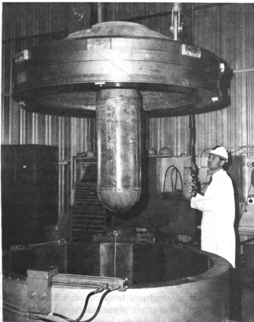
Figur 2 – A concrete test cylinder, instrumented with strain gages, about to be lowered into the 76-inch pressure vessel at CEL's Deep Ocean Test Facility
