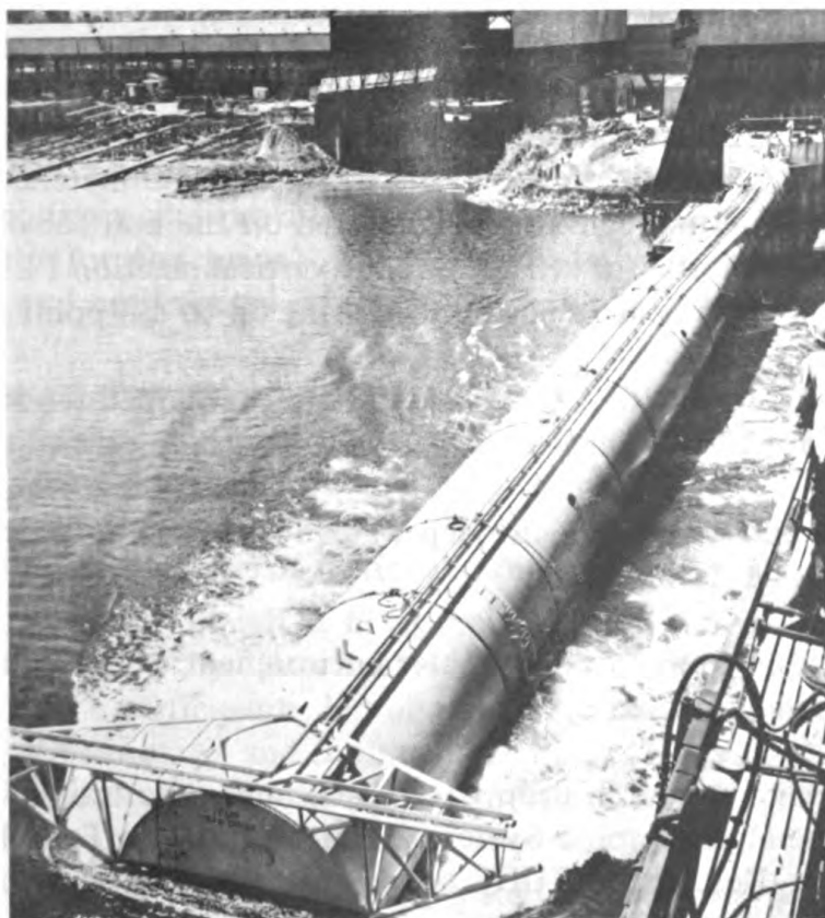
Figure 1 – FLIP showing the aft 225 feet of the vessel where the ballast tanks are distributed
