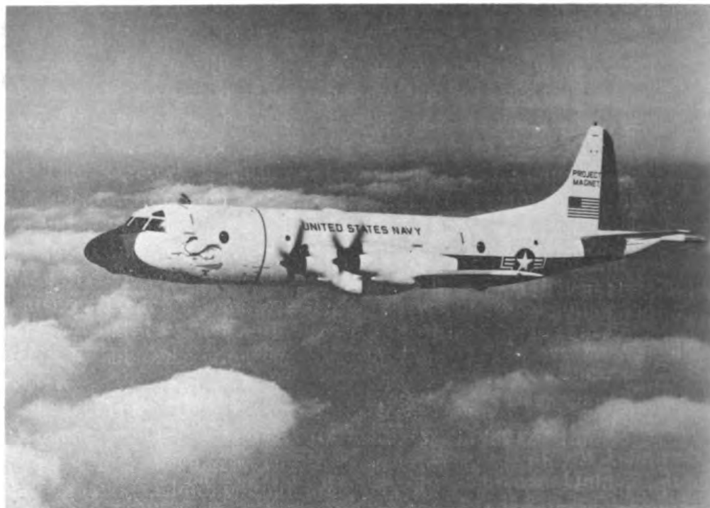
Figure 3 — Project MAGNET's RP-3D aircraft "Roadrunner" has logged over four million miles of marine magnetic surveys and circled the globe four times
