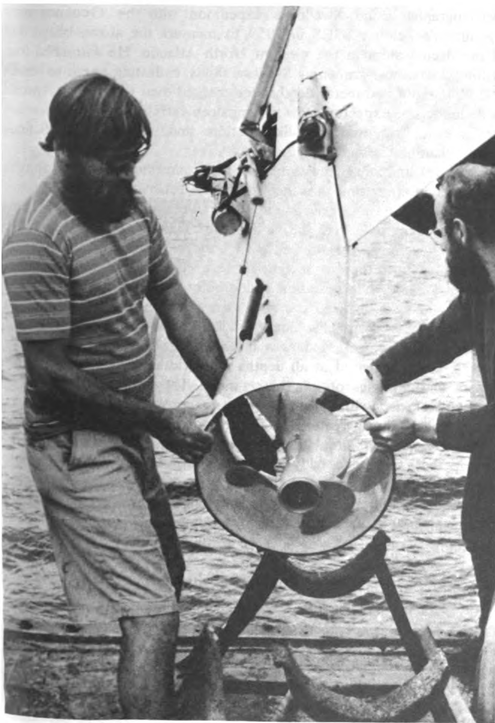
Figure 3 – Launch of towfish during MODE Project aboard CHAIN in 1973. Instrument was used to map density surfaces w/ fine horizontal resolution.
