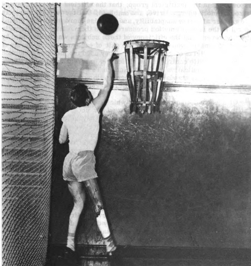
Figure 3. Above-the-knee amputee testing an experimental knee stabilizing device.
