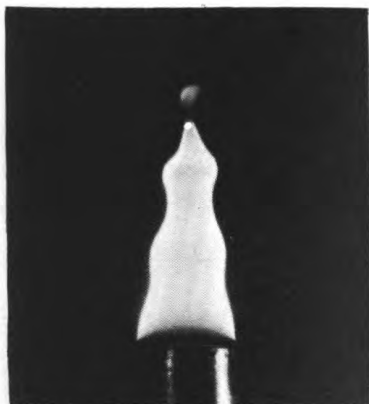
Figure 2. Stroboscopic photograph of Bunsen flame under the influence of an acoustical disturbance.
