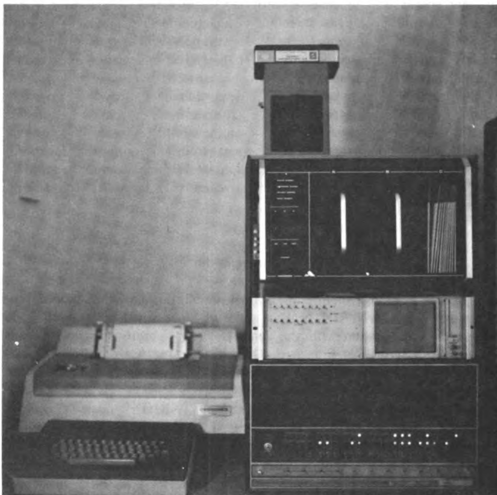
Figure 1 — Computer used in brain wave analysis (right). Cabinet contains the central processing unit, EEG electronics, and floppy disc. Also shown are the keyboard and high speed printer.
