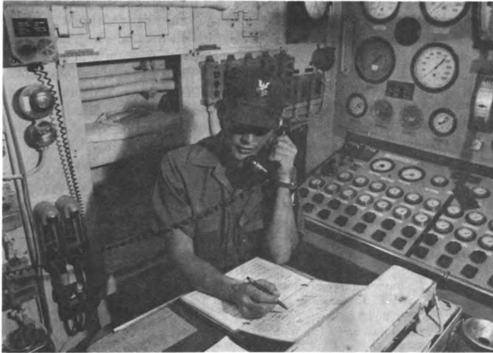
Figure 3 — Boiler Technician follows Engineering Operational Sequencing System diagram in assessing performance of 1200 psi steam propulsion plant.
