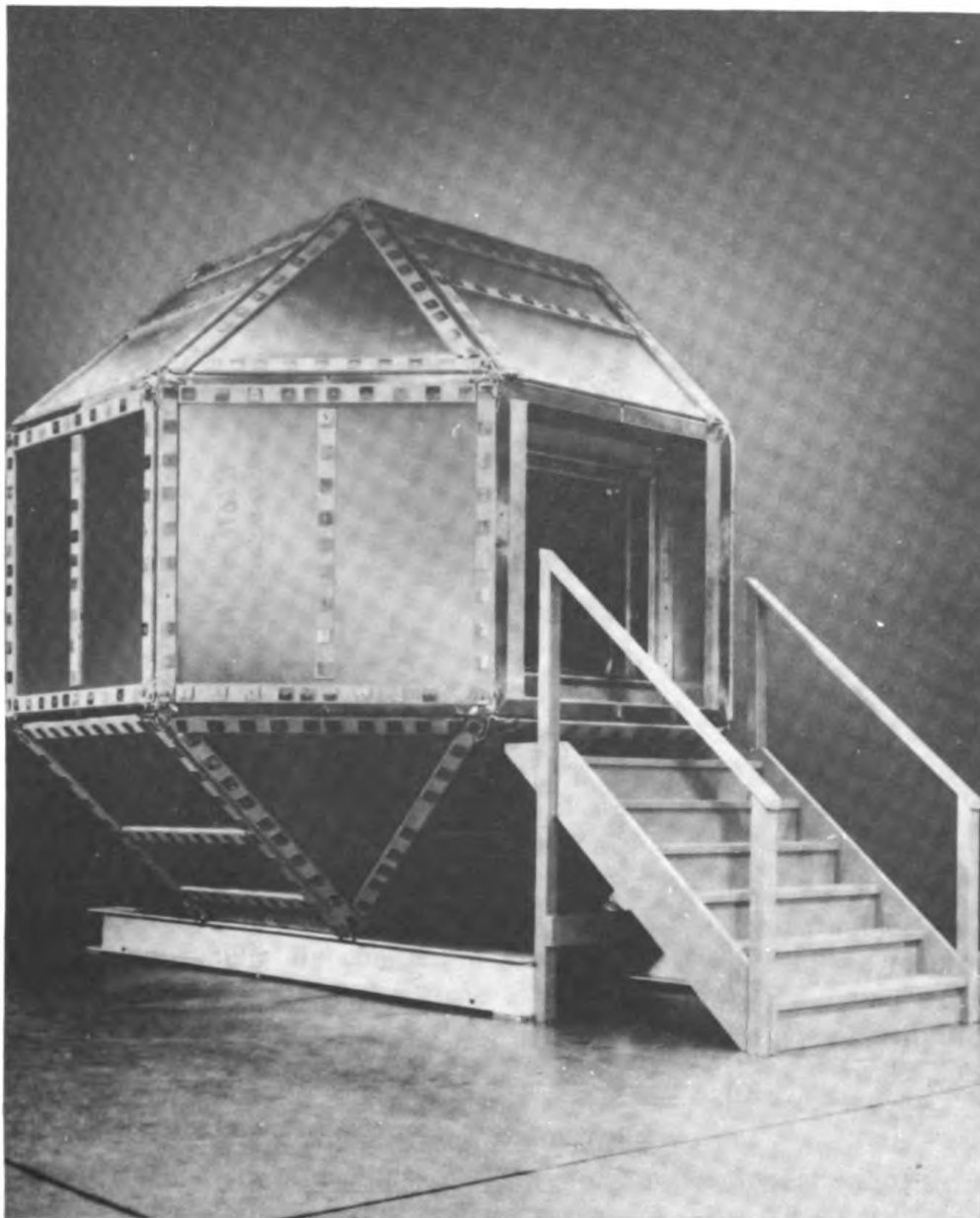
Figure 4 – Magnetically shielded room at the Francis Bitter National Magnet Laboratory at M.I.T.
