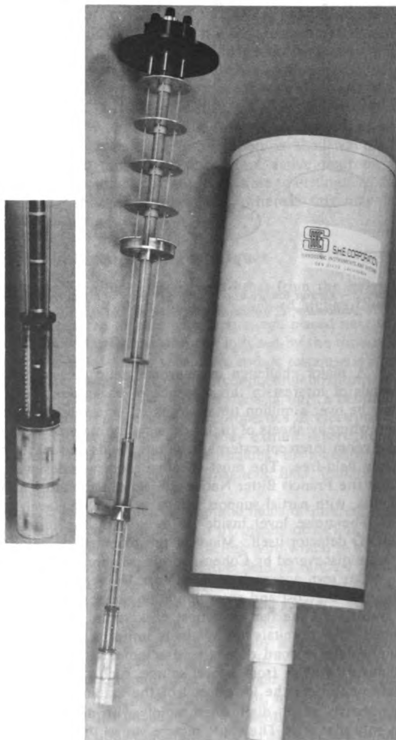
Figure 3 – Supporting structure for a SQUID magnetic field detector displayed beside the cryogenic dewar in which it operates. The SQUID is inside the cylindrical shield located about one-third of the way up the 70 cm long supporting rod. At the bottom is the second derivative gradiometer sensing primary, shown in larger scale in the inset, consisting of niobium wire wound on a 2.4 cm diameter quartz form. (Photographs courtesy of S.H.E. Corporation, San Diego, California).
