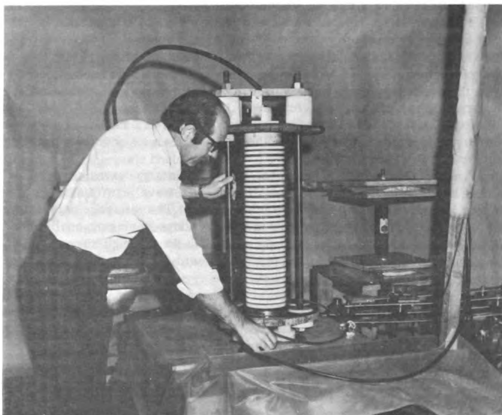
New high power interrupting switch
